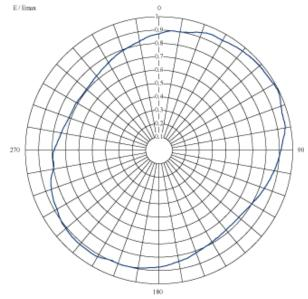
Horizontal Radiation Pattern for Horizontal and Vertical Polarization
