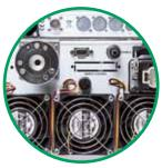
Hot-plug fans: 5 minutes maintenance time, no need to open or switch off the unit.
